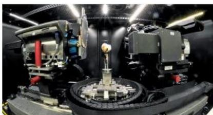
We use X-rays to non-destructively inspect the three-dimensional distribution of matter inside the object of investigation.
