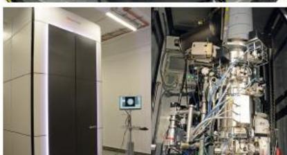
We investigate our samples using high-energy electron beams to obtain images with resolution down to the atom scale.
