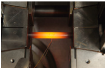
Fig.1: Thermal and mechanical testing of a 100Cr6 test specimen inside the Gleeble 3500.
